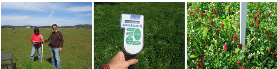
Fig. 3 Electronic capacitance probe Grassmaster II in experimental field tests
