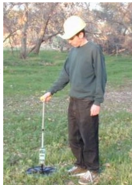
Figure 5—Jenquip Filips folding plate pasture meter.
