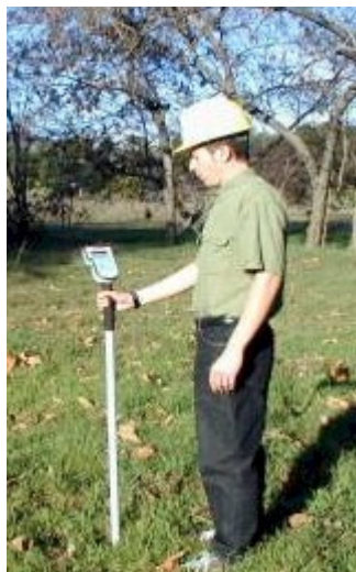
Figure 2—Typical capacitance probe.
