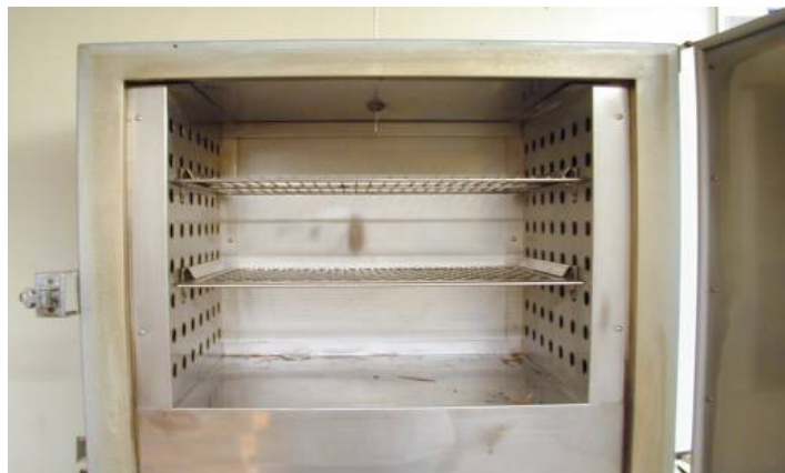
Figure 11—Typical standard mechanical oven used for cut and weigh method.
