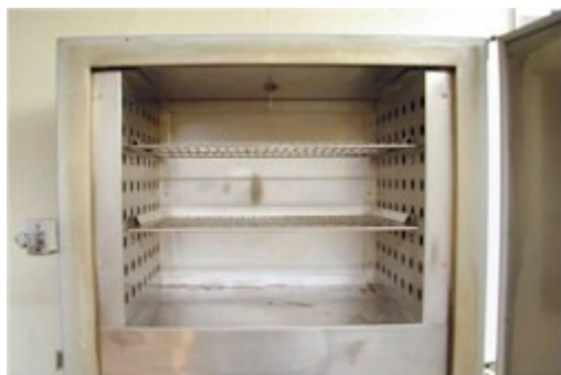
Figure 4—Mechanical convection oven used for cut and weigh method.
