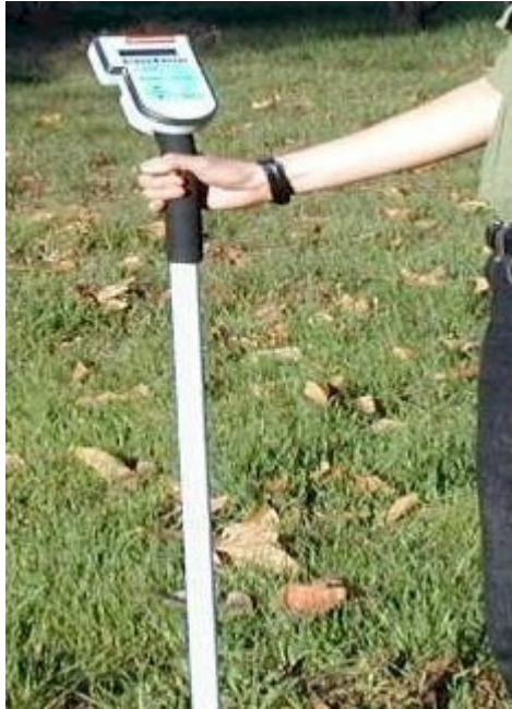
Figure 9—Tru-Test® Limited GrassMaster Pasture Meter.
