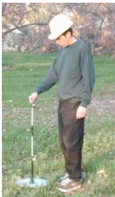
Figure 6—The Kencove FarmTracker™ rising plate.
